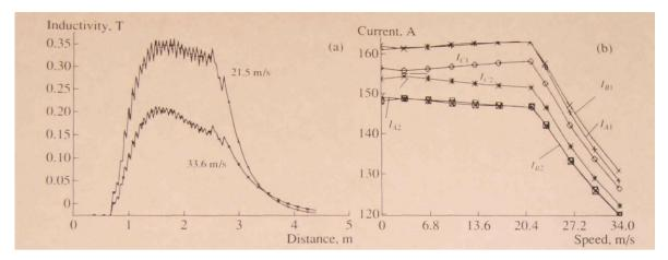
Fiy. 5. Series connection of modules of concentric windings: (a) is the induction distribution along the gapping at a speed of 21.5 and 33.6 m/s and (b) is the phase currents amplitude variation in the velocity function.
